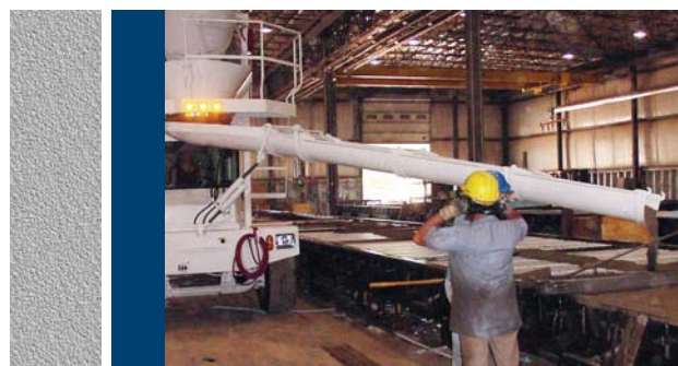
Placing concrete inside plant using Indiana Phoenix's new pre-cast concrete delivery machine. Eliminating features from standard machines that pre-casting doesn't require can save massive amounts of time and cost.
